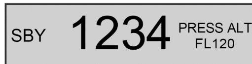
Figure 5: Pressure Altitude screen
